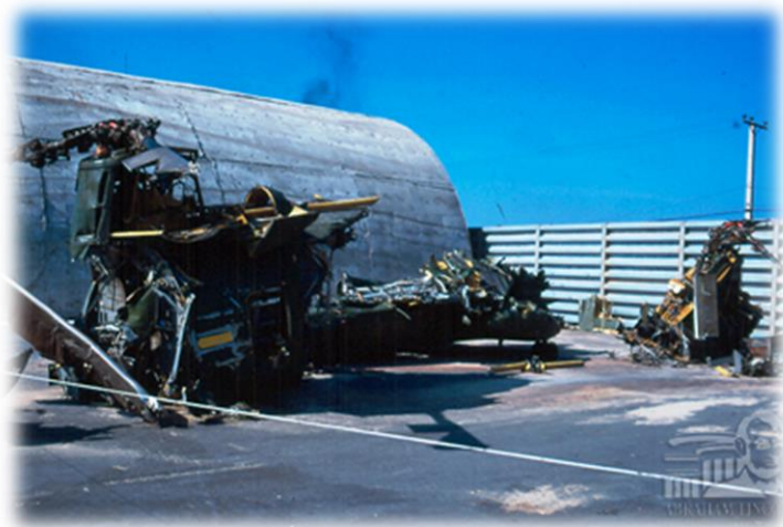
The remnants a CH-46 Sea Knight helicopter, following seizure of the forward transmission and de-syncing of the rotor systems. The helicopter crashed in front of the officer's club at Marble Mountain in the spring of 1971.
